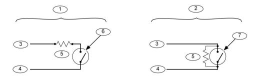
Figure 3.8: Keyswitch Wiring
